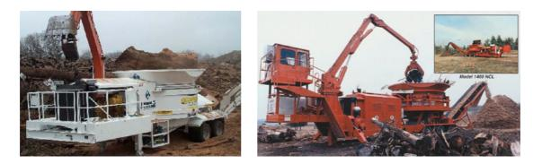
The equipment can be operated by one operator and uses a high speed grinding design to quickly reduce waste (drive engine power 1.5kW - 300kW)..
