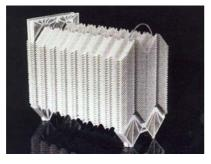
The use of a coalescing plate separator is appropriate for oily water streams with relatively low particulate impurities. The units are able to handle low to medium flow ranges. For larger flow rates, a modular design is applied i.e. several smaller units operate in parallel.
